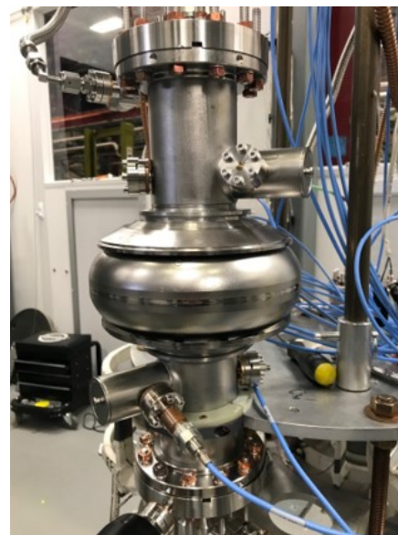
Figure 7: Single cell cavity equipped with higher order modes couplers.
