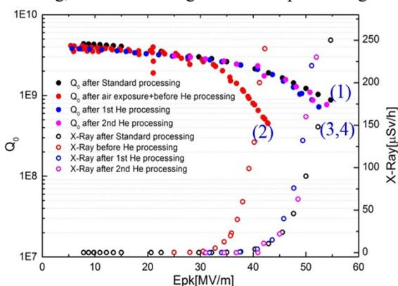
Figure 4: The test results of the HWR015 cavity, after standard surface processing (curve (1), black circles); after air exposure, baking(120<sup>0</sup>C for 58 hours), and Ar/O2 plasma cleaning (curve (2), red circles); after helium processing (curve (3,4), blue and pink circles).
