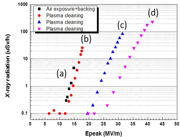
Figure 3: The X-ray test results of the HWR015 cavity experienced air exposure and baking (curve (a)) and plasma cleaning (curve (b), (c), (d)).
