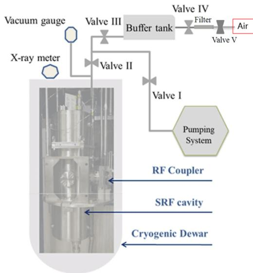
Figure 1: The experimental schematic of air pollution for HWR015 cavity.
