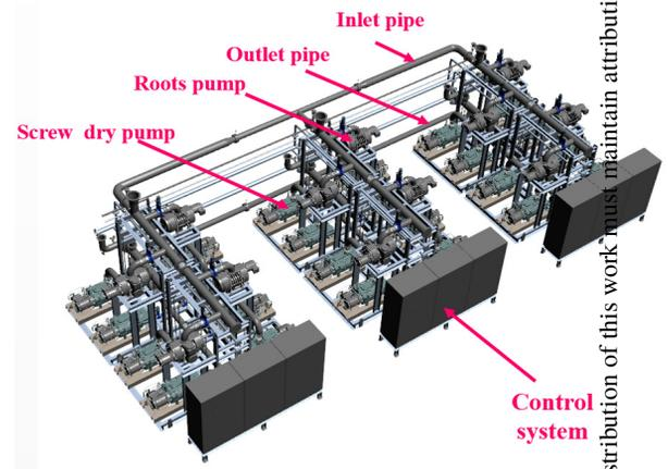
Figure 8: Three-dimensional diagram of 2K vacuum pumps system.
