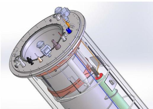
Figure 3: Three-dimensional structure of vertical test cryostat.
