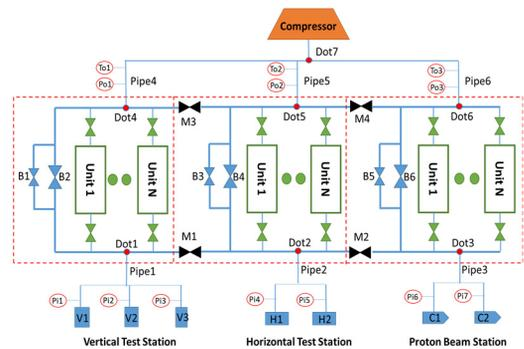
Figure 7: Faction diagram of 2K vacuum pumps system.
