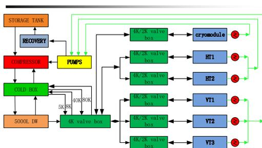
Figure 1: Flow chart of the helium cryogenic system of the PAPS.
