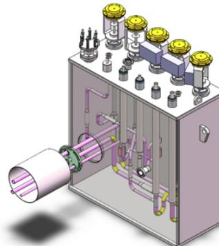
Figure 4: Three-dimensional structure of cryogenic distribution valve box.
