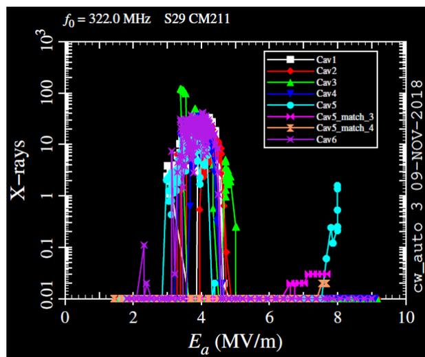
Figure 2: SEL High Power Test Ea vs. X-ray (SCM211).
