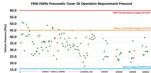
Figure 7: FRIB HWRs Pneumatic Tuner Requirement Pressure for Specification Frequency at 2K (until April 2019).
