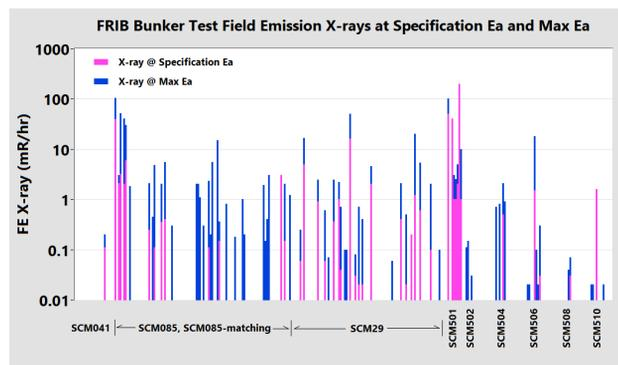
Figure 9: FRIB Cryomodule Bunker Test (until April 2019), Field Emission cavity X-rays at Specification  $E_a$  and Max  $E_a$ .
