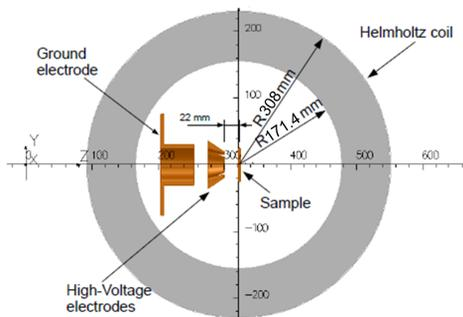
Figure 4: The four-segmented electrode in front of the sample used for both deceleration and high magnetic field compensation (modified from [6]).
