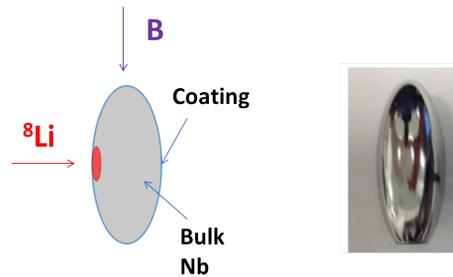
Figure 5: Heat treated ellipsoid samples planned for incoming beamtime with the modified zero/low-field spectrometer.
