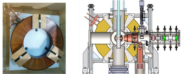
Figure 6: Left: Helmholtz coil received on-site, which has been fabricated and qualified by Stangenes Industries. Right: Design of coil bracket and support for Phase-II installation.
