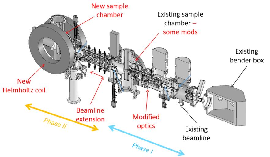
Figure 2: Scope of  $\beta$ -SRF project for phase I (modified) and phase II (new).
