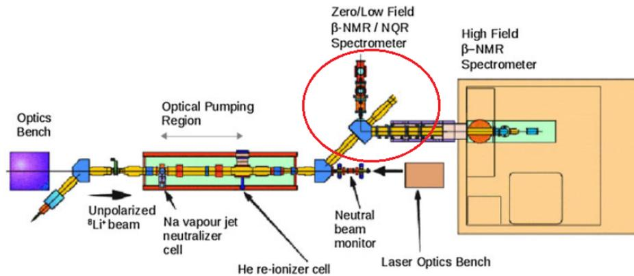
Figure 1: Current  $\beta$ NMR beamline with two spectrometers at different magnetic field ranges [5]. Beta-SRF facility is designed as an upgrade to the zero/low-field spectrometer circled in red colour.
