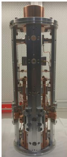
Figure 3: Modified beam optics after clean-room assembly.
