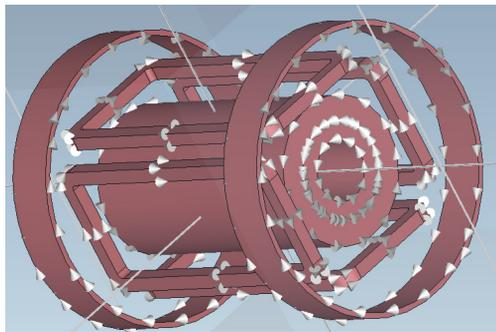
Figure 6: 50 cm solenoid package modelling for CST.
