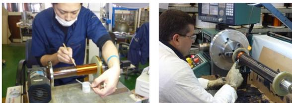
Figure 8: Solenoid winding, dry winding at KEK (left), and wet winding at MSU (right).
