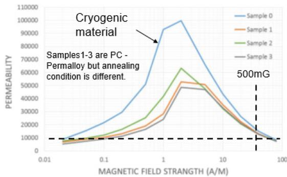
Figure 11: Field dependence of permeability at 20 K.
