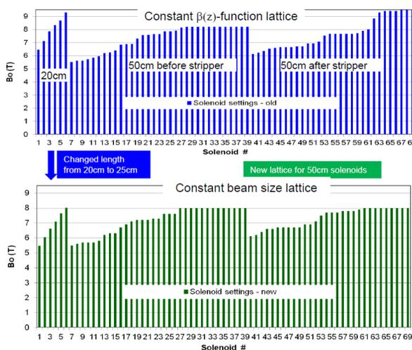
Figure 2: FRIB beam optic change from the constant beta scheme to constant beam size, which reduces the solenoid field from 9 T to 8 T.
