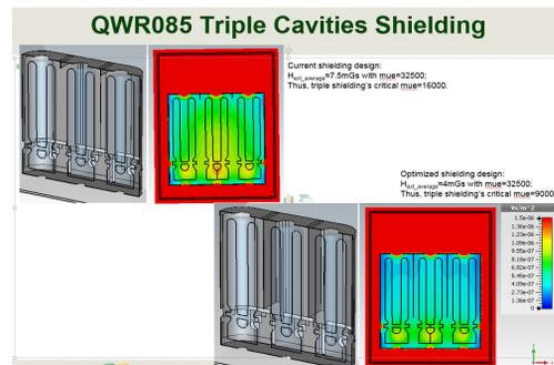
Figure 12: Example of magnetic shield optimization, 0.085QWR CM case. If add plates between cavities,  $\mu=9000$  meets the FRIB requirement ( $< 15$  mG in the shield).
