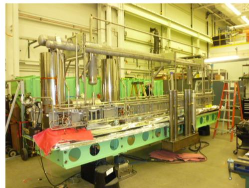
Figure 10: Coldmass on the cryomodule baseplate for the local magnetic shield design validation. Two cavities surrounded magnetic shield and one solenoid are seen.
