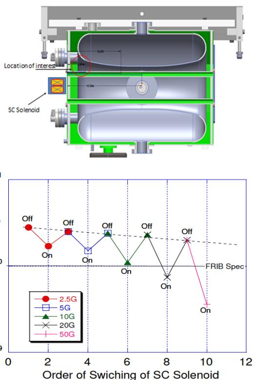
Figure 4: HWR cavity quench test operating solenoid. The cavity was quenched under a solenoid field and confirmed Q-drop (bottom).
