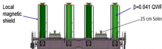
Figure 1: FRIB cryomodule design example for 0.041QWR coldmass. Two SC magnet packages and local magnetic shield around cavity are seen.
