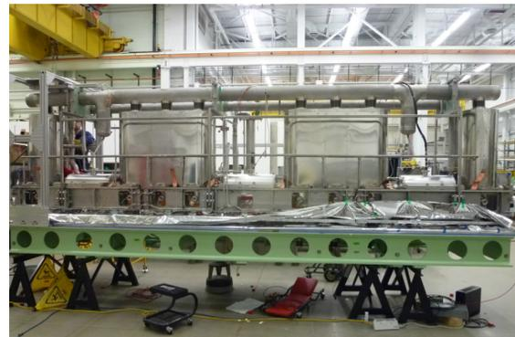
Figure 13: FRIB first 0.085QWR production cryomodule. In the left (one cavity and other three cavies group) in the mirror symmetry PC Permalloy was used and right Mu-metal was used for magnetic shield material.
