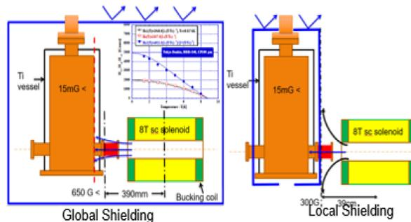
Figure 3: Cavity fringe field exposure during solenoid operation, left (Blue Square) is the global magnetic shield and right local shield (blue square).
