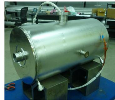
Figure 9: 50 cm solenoid package coldmass (left) with the stacked diodes for quench protection. A completed 50 cm solenoid package at MSU with dressed stainless helium jacket (right).
