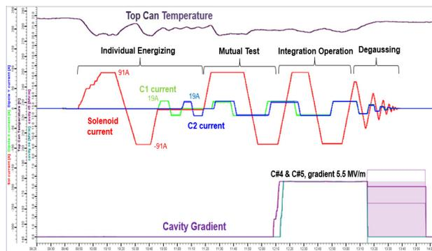
Figure 14: Solenoid package bunker test example (0.53HWR CM). All magnets were co-operated at the maximal field with cavities at operation field, all magnets were changed polarity. No quench happened. Solenoid package is very stable and robust.
