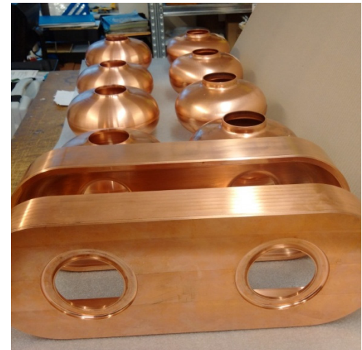
11-cell copper cavity parts ready for completion
