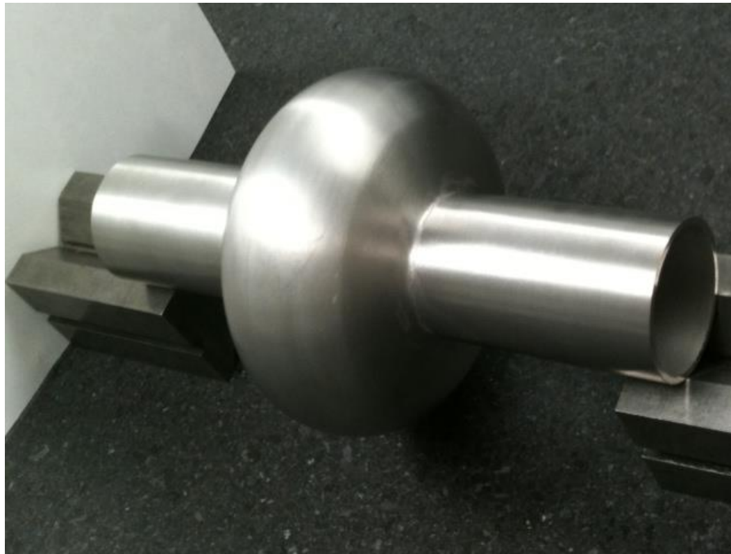
CVD niobium cavity after machining
