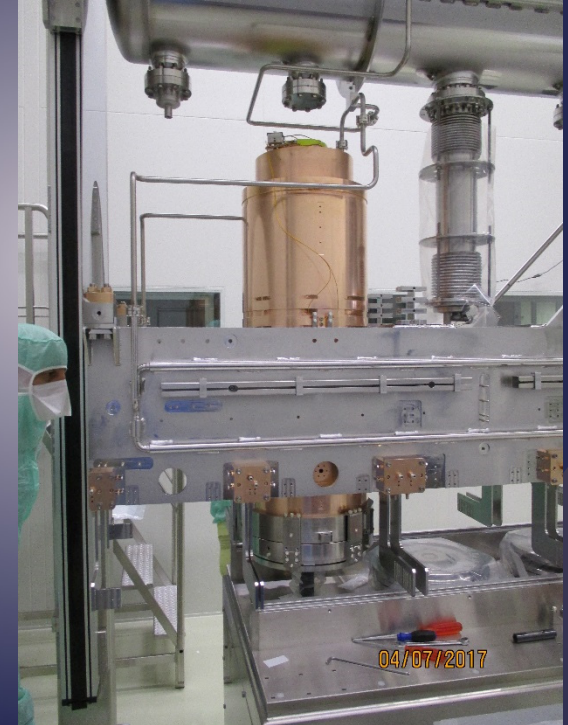
Blank assembly of a seamless cavity, July 2017
