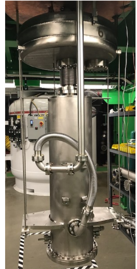
Beta=0.85 QWR hanging on vertical test insert the day after a vertical test
