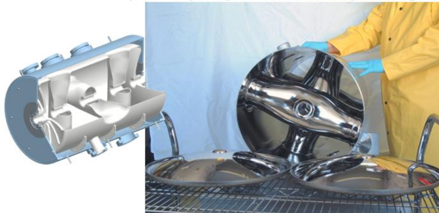
\beta=0.5 Triple-Spoke after electropolishing
