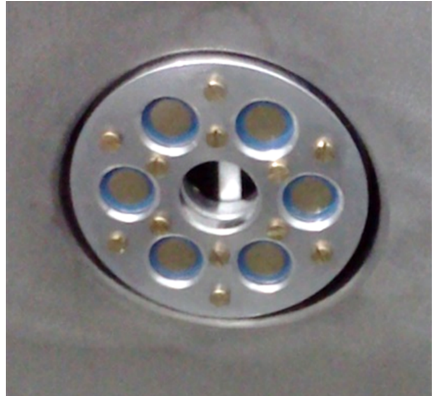
52 mm, 6-channel multi-OST in a helium tank of the cavity
