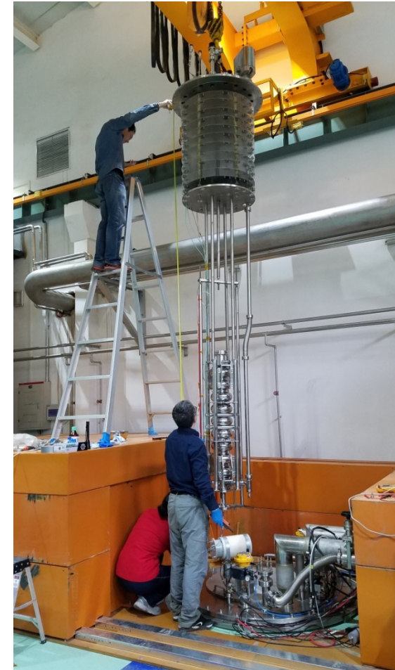
Vertical test of 6 large grain 9-cell cavities (April ~ June, 2017)
