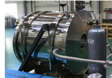
HTS (High Tc Superconducting) Magnet
