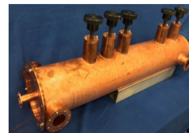
Harmonic Fast kicker for cooling ring
