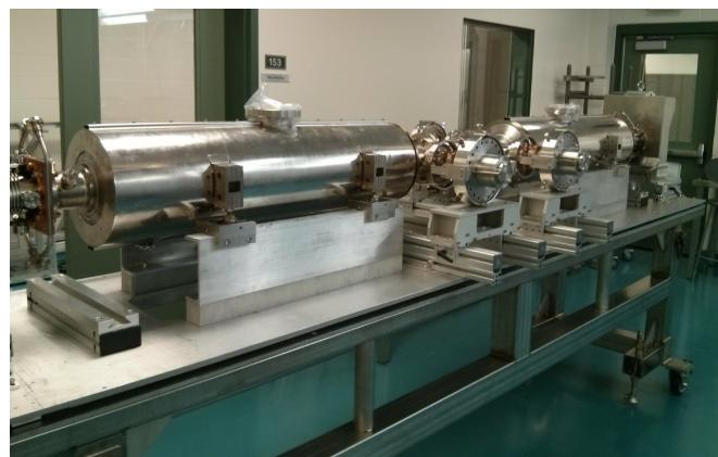
Hermetic unit re-installed on cold mass top assembly and the cryomodule (now ACMduo) was moved to the e-hall March 2017 for installation in April 2017
