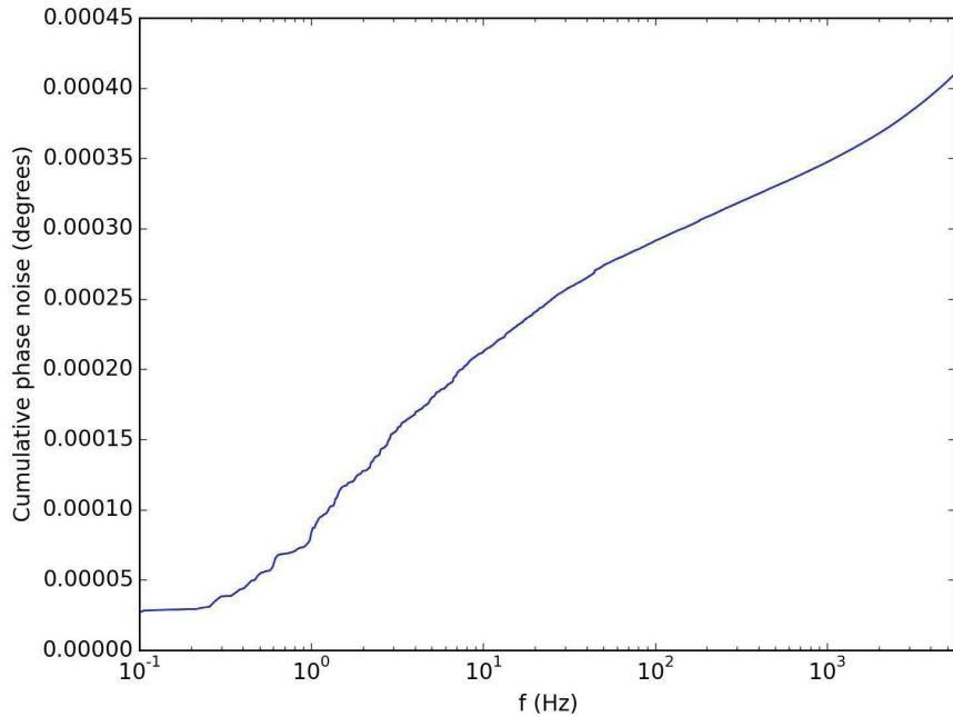
Note 1 Hz high-pass included to represent beam-based feedback and to avoid logarithmic singularity of  $1/f$  noise integral to DC.
