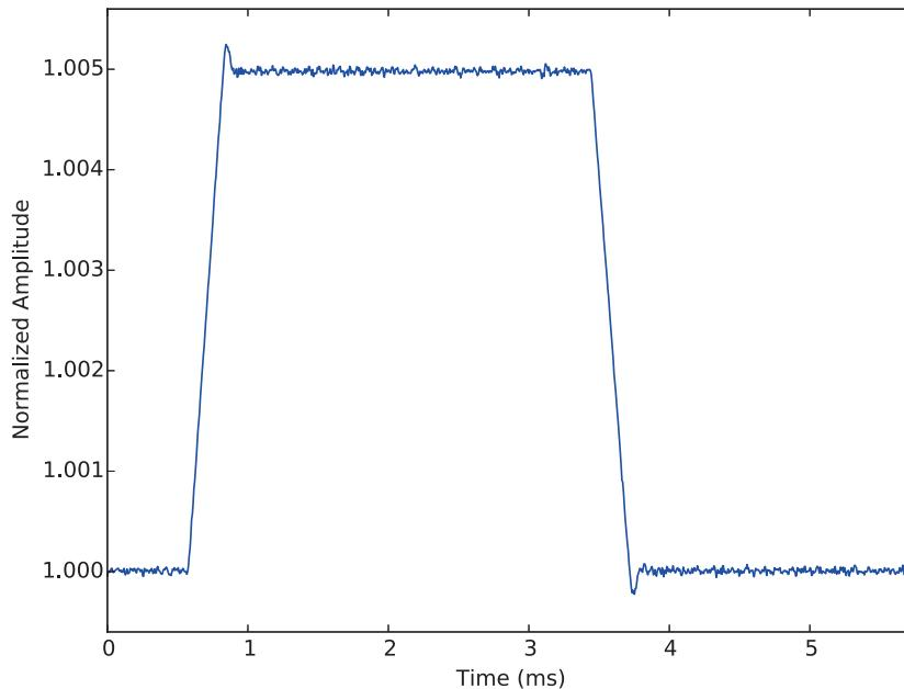
Response to 0.5% amplitude step in setpoint, slew-rate-limited due to clip limits and cavity pole.
