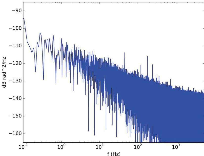
Measured at 1300 MHz using passive splitter and short cables to two Rx inputs.
