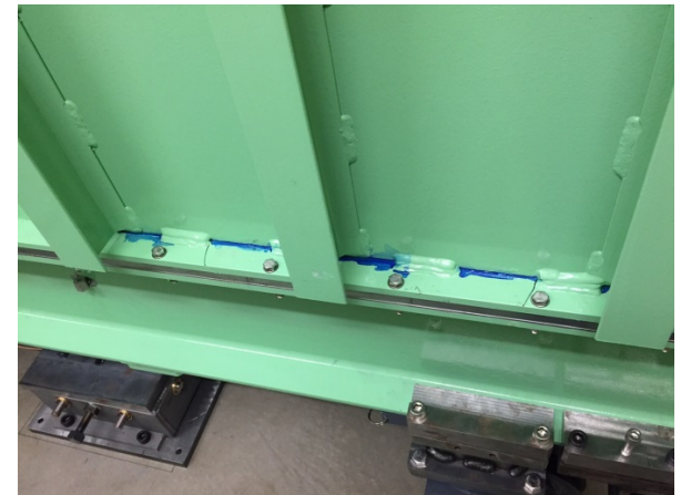
\beta=0.53 cryomodule vacuum vessel welding defect
