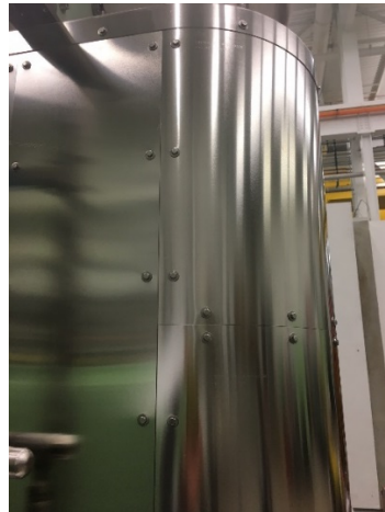
Magnetic shields using fasteners for assembly
