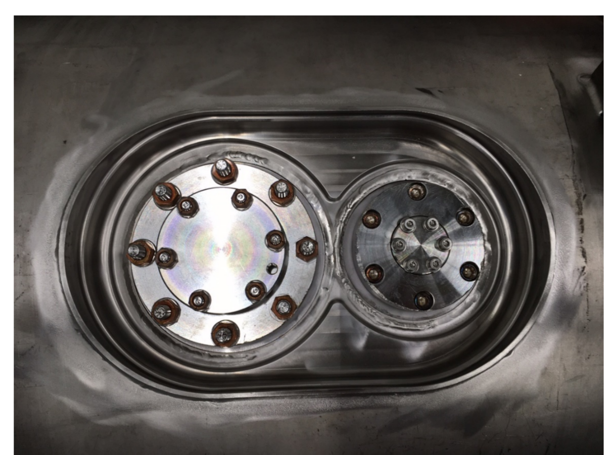
Trough profile as replacement for the leak bellows.
