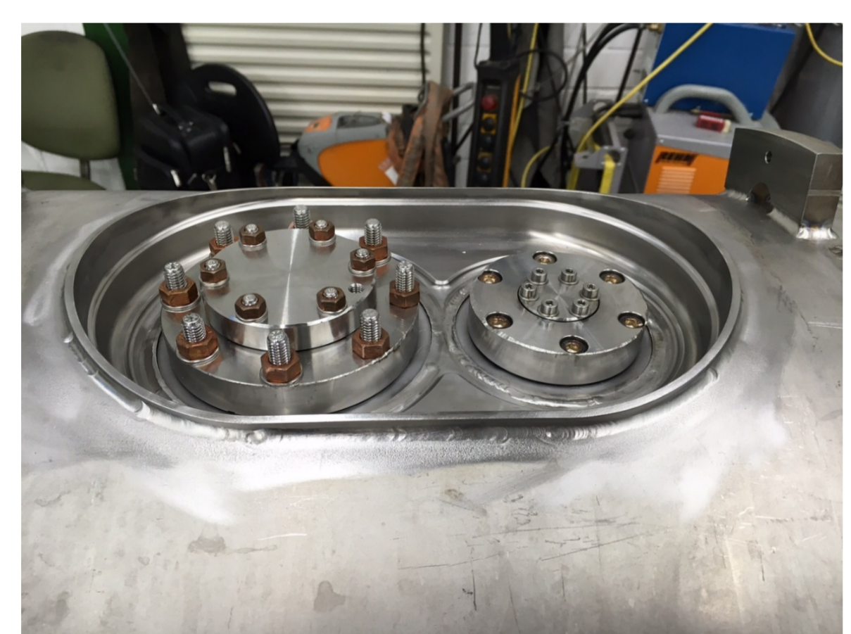
Trough profile as replacement for the leak bellows.
