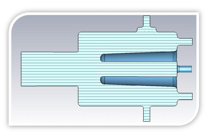
The figure shows the RF model of the recently designed 166.6 MHz cavity namely PoP cavity.
