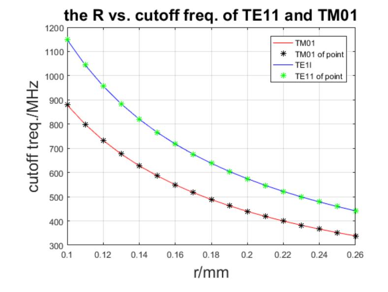
Damping all HOMs from enlarged tube, the radius of the tube needs at less 260mm.
