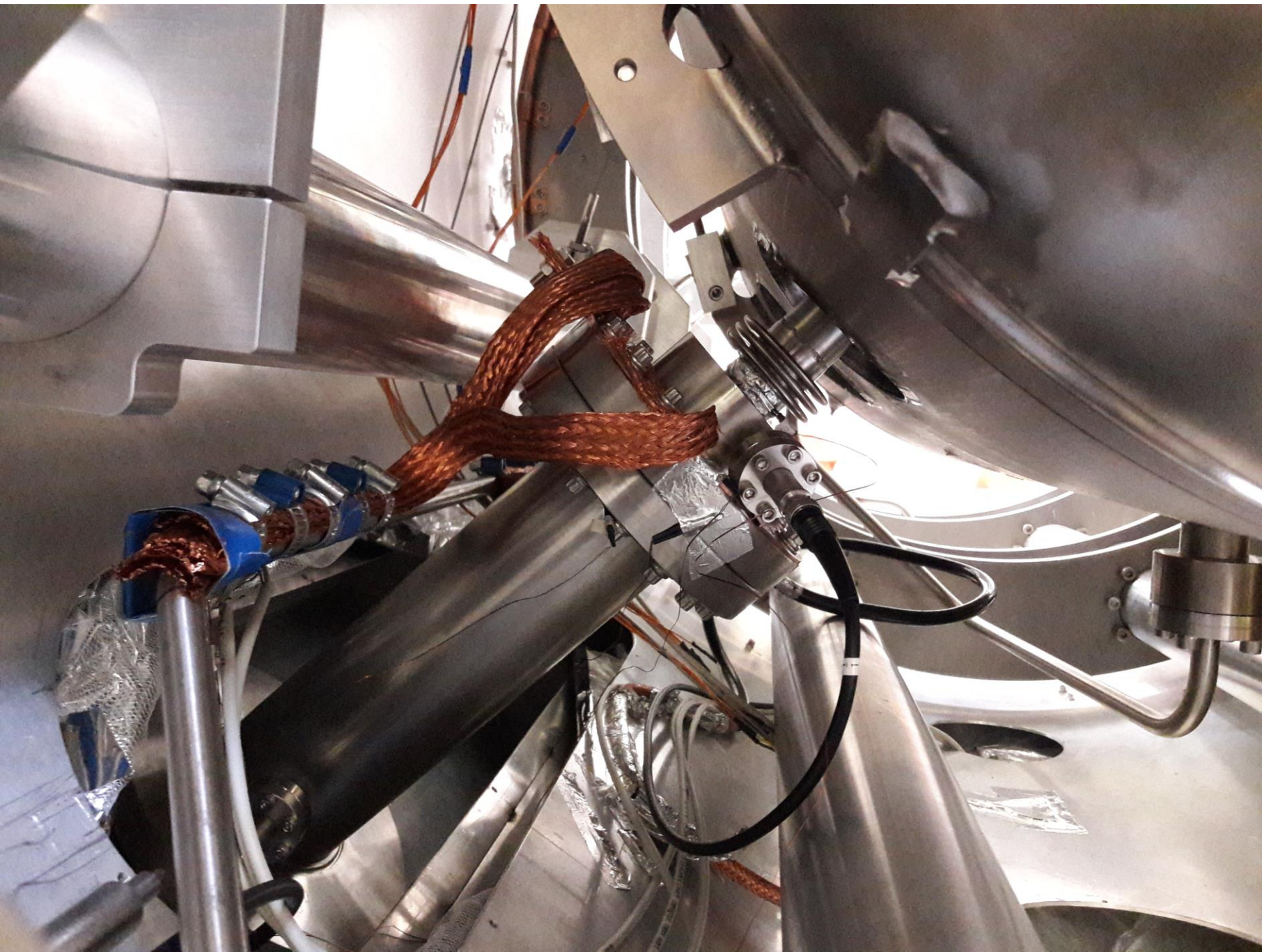
5 kW power coupler assembled to cavity and cryostat
