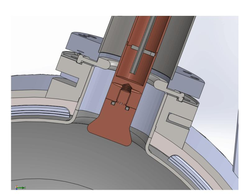
Solution of CM1: Both special gasket and enlarged antenna tip were designed to shield the FE.
