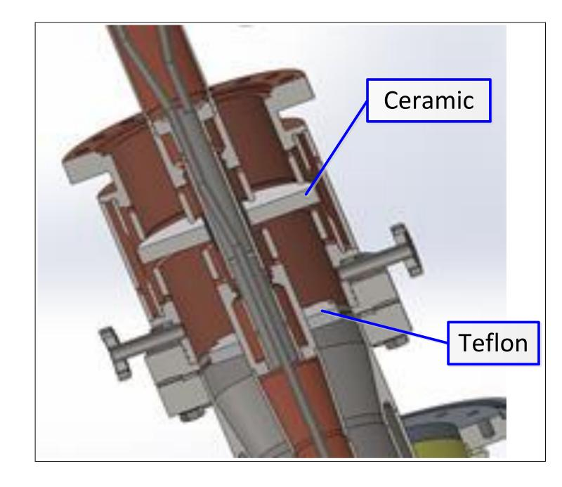
A piece of Teflon plate were put into the area between the ceramic and the coupling port to barrier the FE electrons. We found that the ceramic never cracked after Teflon plate shielding.
