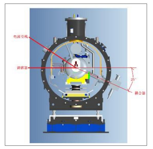
The cross section of and CM4: coupler position downside
