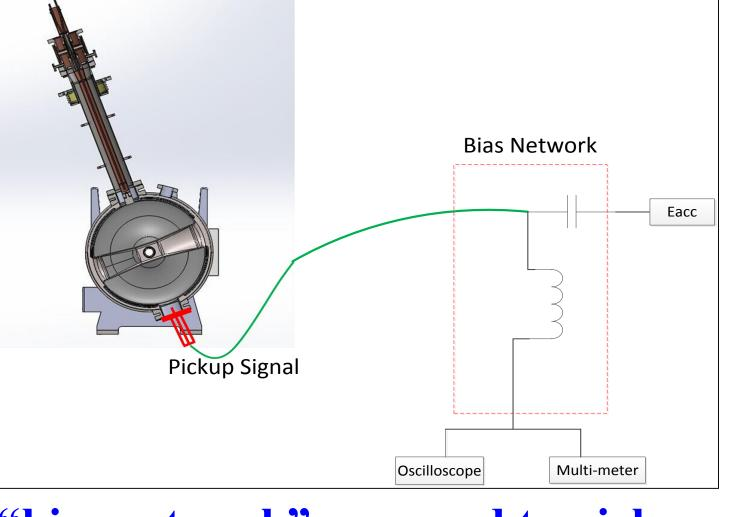
A "bias network" was used to pick up the DC voltage from the pickup port.
