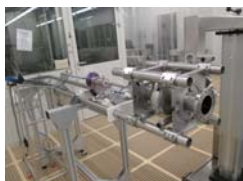
Connection of cavity to inspection device, horizontal adjustment partly possible
