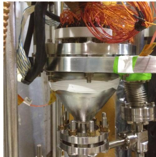
Figure 6: The Cornell Sample Host Cavity. The sample plate is at the top of the cavity with a temperature mapping system attached to it.
