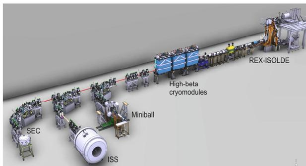
Figure 1: Layout of the HIE ISOLDE linac in 2017.
