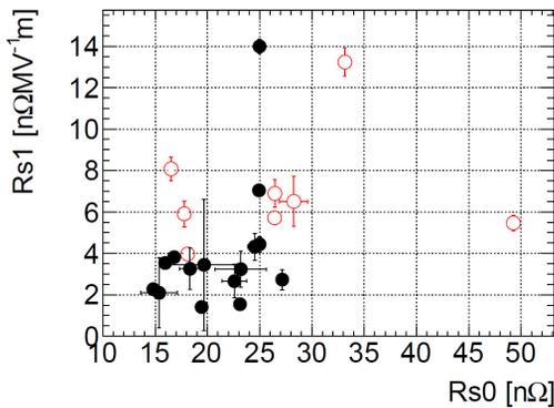
Figure 6: correlation between defects and performance. Empty symbols denote cavities with defects on substrate.
