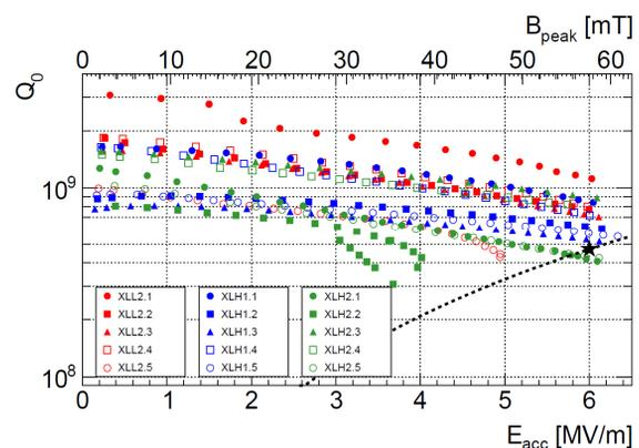
Figure 2: on line performance of the first 15 cavities. The dotted line corresponds to 10 W cavity power dissipation.
