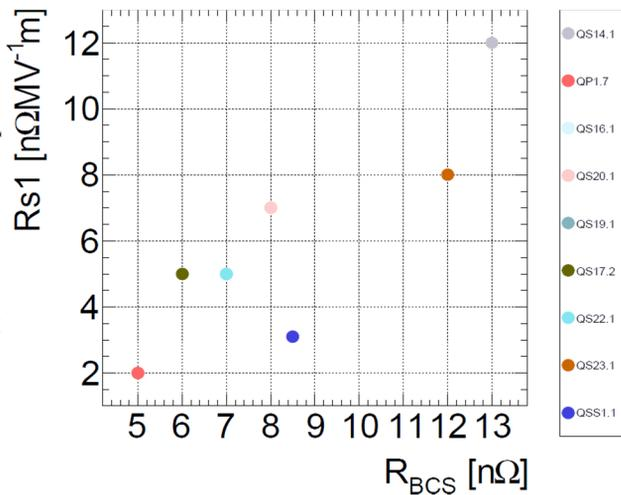
Figure 9: linear Q-slope vs the apparent RBCS.
