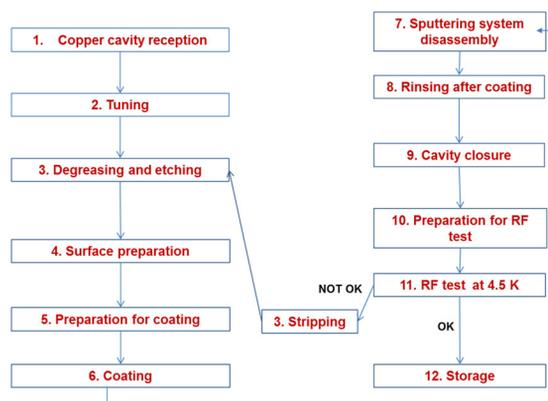
Figure 3: Cavity production workflow at CERN.
