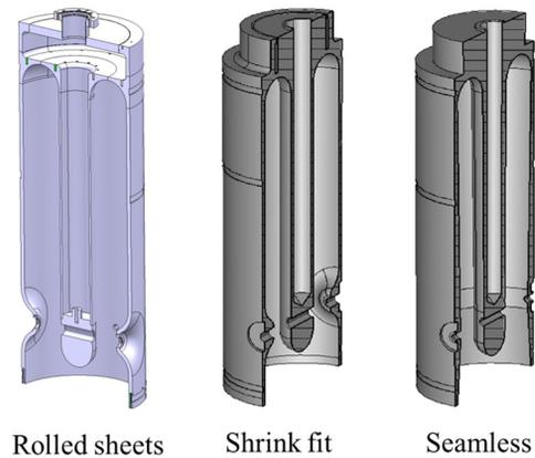
Figure 4: Evolution of cavity design.
