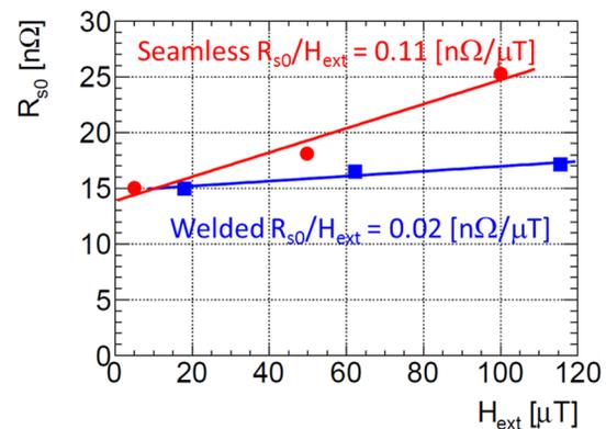
Figure 8: Sensitivity of two HIE-ISOLDE cavities to trapped flux.
