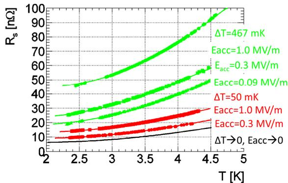
Figure 7: dependence of  $R_s(T)$  on field levels and on temperature gradient upon cool down.
