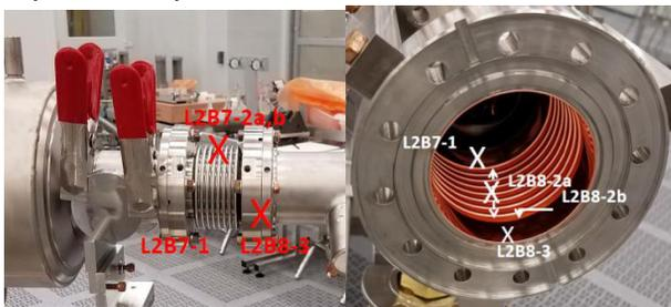
Figure 5: LCLS-II bellows sampling locations.
