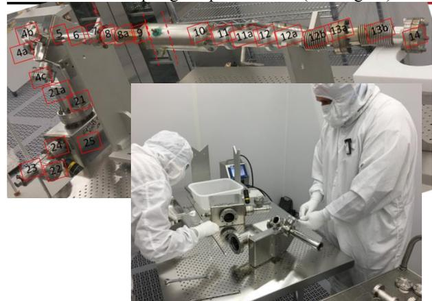
Figure 2: CEBAF beamline girder during particulate sampling in cleanroom.
