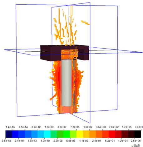
Figure 7: The calculated prompt dose rate distribution during testing a TESLA 9CELL cavity.
