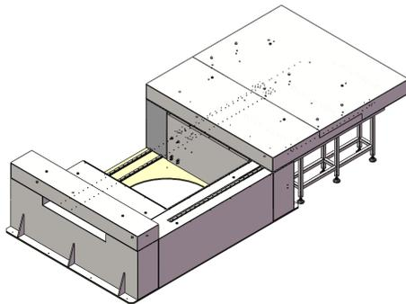
Figure 6: The external radiation shielding.
