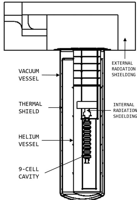
Figure 1: Layout of VTS and cryostat.
