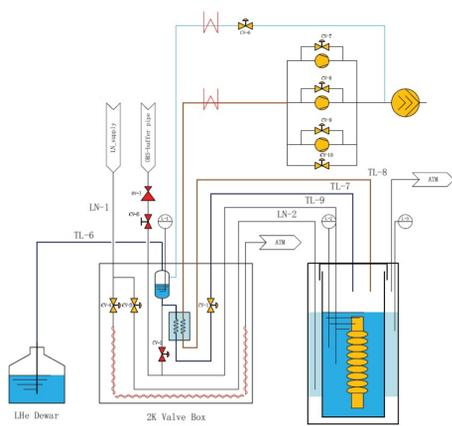
Figure 3: Schematic diagram of the 2 K system.
