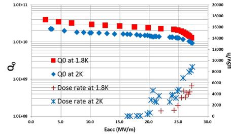
Figure 10:  $Q_0$  and radiation level with respect to the  $E_{acc}$  in the commissioning trial.
