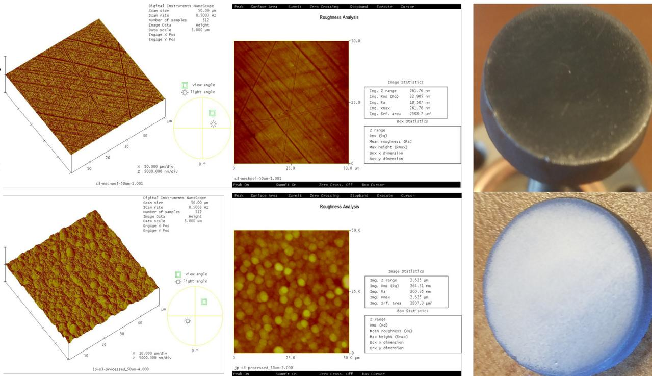
Figure 3: Top: AFM scan, roughness profile, and photo before plasma etching. Bottom: AFM scan, roughness profile, and photo after plasma etching.
