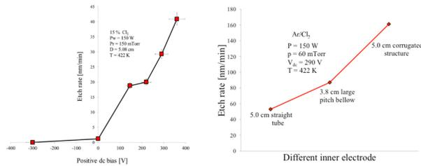
Figure 1: Left: Etch rate vs. dc bias. Right: Etch rate vs. electrode geometry.
