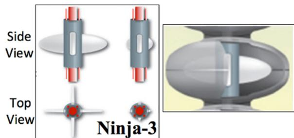
Figure 1: Schematic view of Ninja cathode (with 4 insulating wings and enhanced cathode area, Ninja-3).
