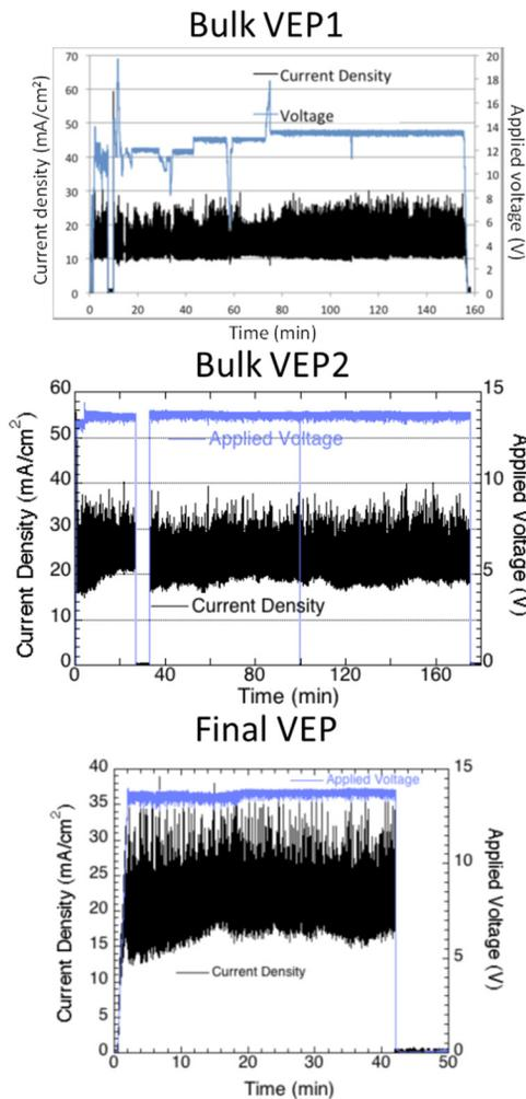
Figure 3: Logged data of voltage and current density of each VEP (Upper: bulk VEP1, Middle: bulk VEP2, Lower: final VEP).
