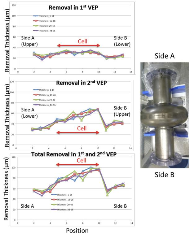
Figure 4: Removal thickness distribution after each VEP (Upper: after bulk VEP1, Middle: after bulk VEP2, Lower: total of bulk VEP1 and bulk VEP2).
