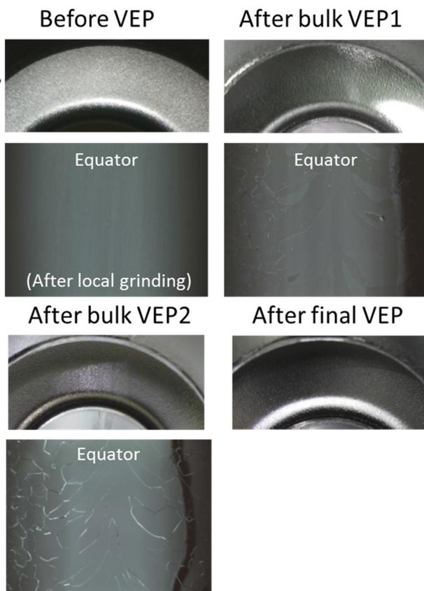
Figure 5: Surface inspection results before and after each VEP (Upper: digital camera, Lower: Kyoto camera).
