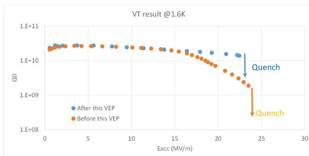
Figure 6: Vertical test result before and after this VEP (Blue dots: after this VEP, Orange dots: before this VEP)
