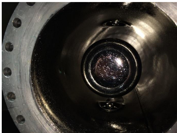
Figure 2: RF surface of QWR # I03 post EP accident.
