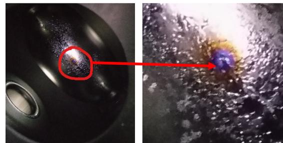
Figure 3: Bluish violet spot on the surface of inner conductor.
