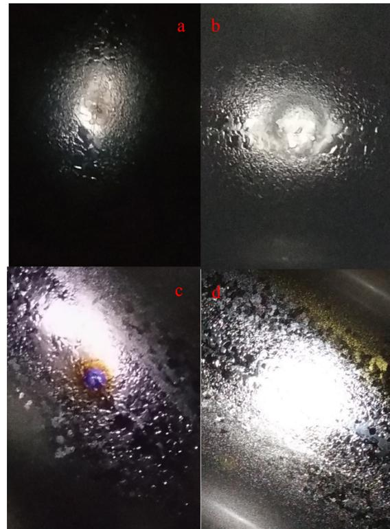
Figure 6: Surface recovery of the cavities inner conductor.
