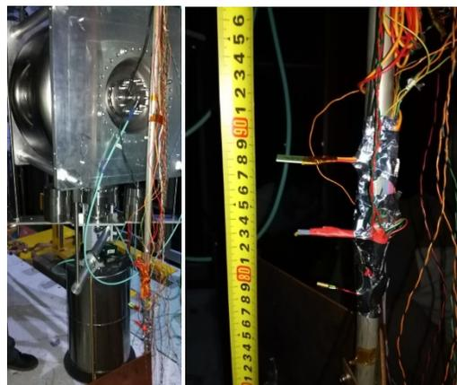
Figure 6: Position of second sound detector with spoke cavity.
