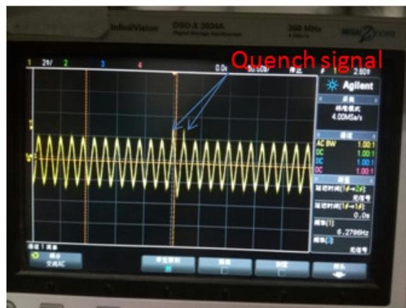
Figure 5: Second sound signal of QWR cavity.
