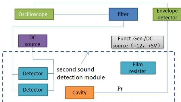
Figure 3: Circuits of second sound detection experiments in liquid helium.
