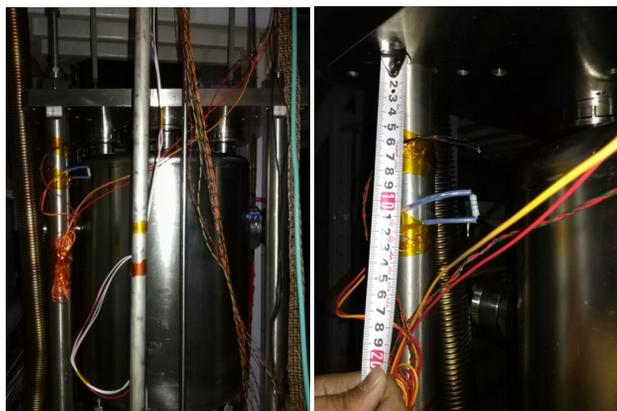
Figure 4: Position of second sound detector with QWR cavity.
