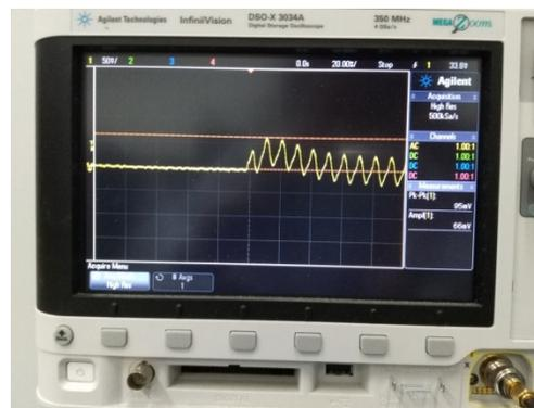
Figure 7: Second sound signal detected by germanium resistor from the film resistor.
