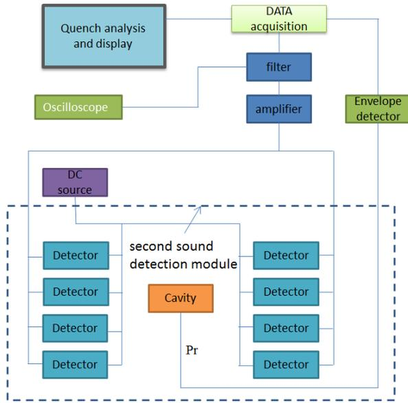
Figure 8: Circuits of second sound detection system of PAPS.
