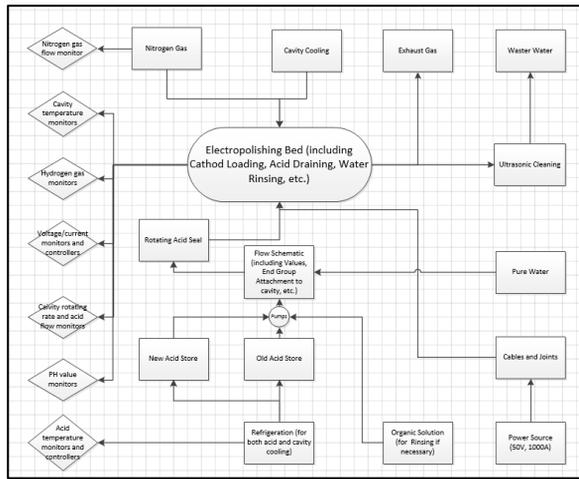
Figure 2: Main components for EP system.
