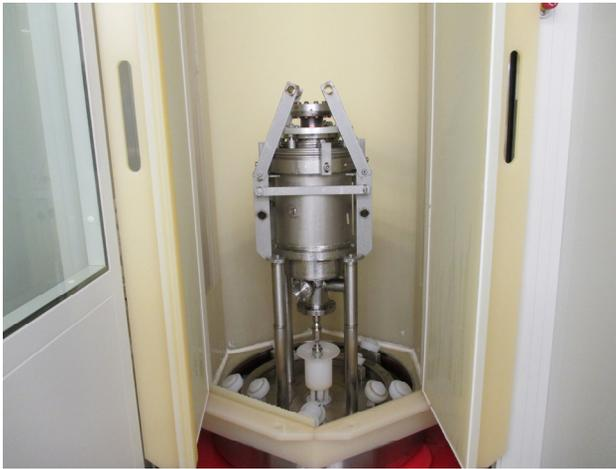
Figure 11: SRF Gun cavity 3RG2 installed to HPR stand.
