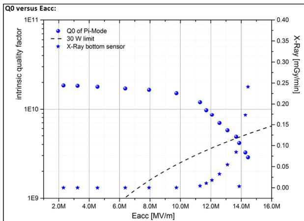
Figure 13: Test result of the SRF gun cavity 3RG2.
