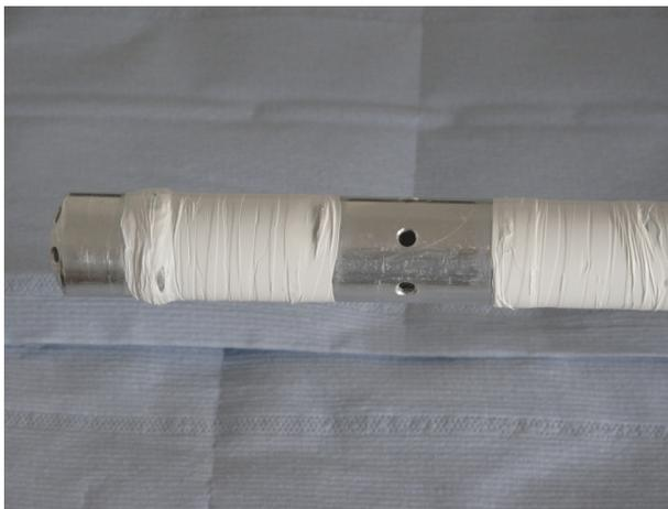
Figure 9: view on acid injection holes and masking of cathode for 1.6 cells SRF gun cavity vertical EP.
