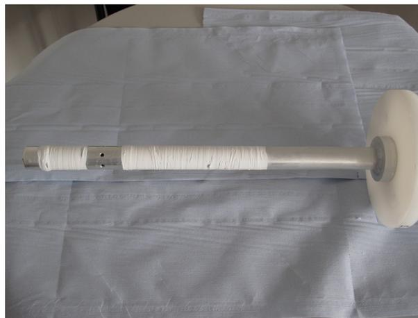
Figure 7: Cathode for 1.6 cell gun cavity EP.
