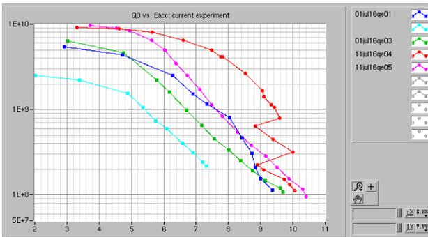
Figure 12: Test results of SRF Gun cavity 16G2 after third vertical EP.
