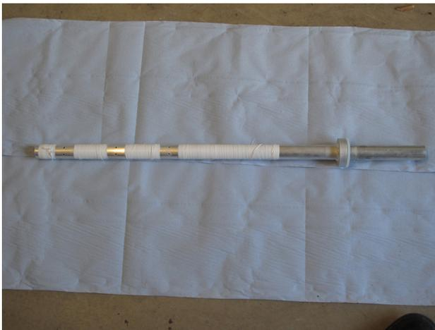
Figure 8: Cathode for 3.5 cell SRF gun cavity EP.
