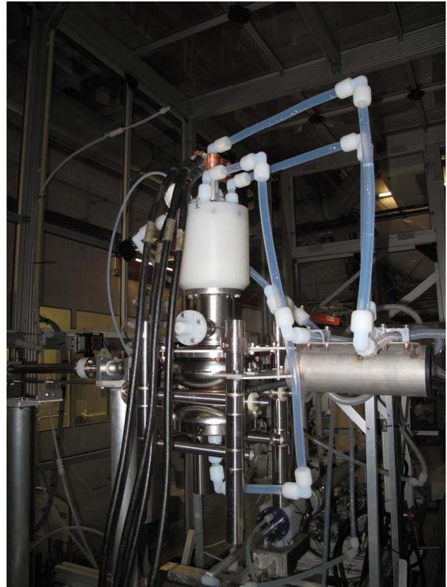
Figure 1: 1.6 cells SRF gun installed in the DESY EP set up.
