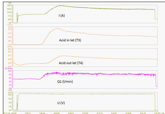
Figure 10: Data of 1st vertical EP on 3RG2
