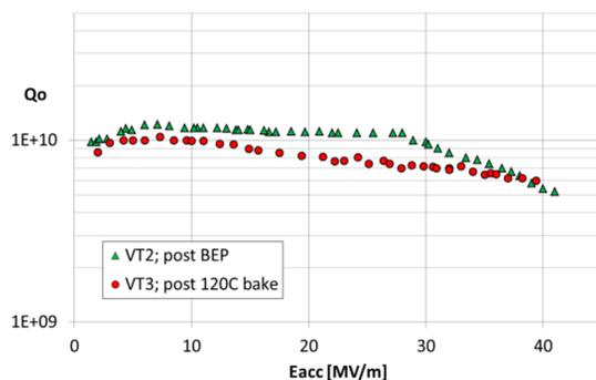
Figure 5: The results of LTE1-14, comparing  $Q_0$  post Bipolar-EP and post 120 °C bake at 2K.
