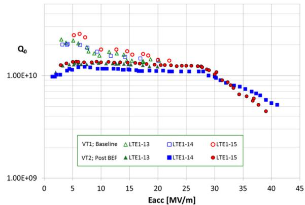
Figure 3: RF test results from the 1<sup>st</sup> and 2<sup>nd</sup> RF test runs at 2K.
