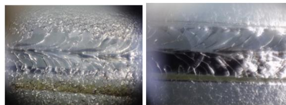
Figure 4: Optical inspection images of the equator weld seam; Cornell VEP (left), Bipolar EP (right).
