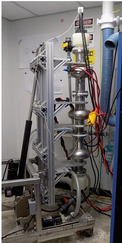
Figure 2: The three 1-cell string on the 9-cell scale Bipolar-EP system at Faraday Tech.
