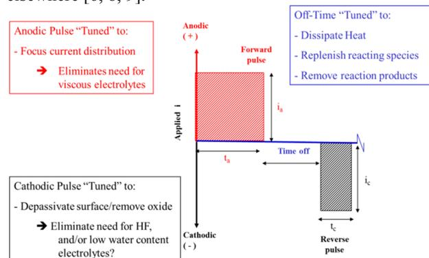
Figure 1: General bipolar EP process representation [6].
