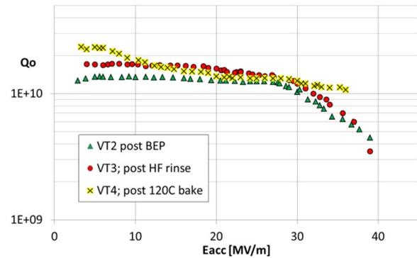
Figure 6: The results of LTE1-15, comparing  $Q_0$  post Bipolar-EP (VT2), post HF rinse (VT3), and post the 120°C bake (VT4) at 2 K.
