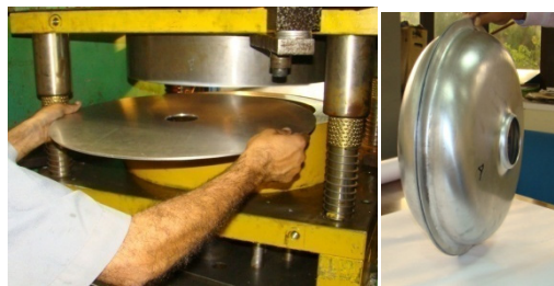
Figure 4: Forming of elliptical half cells.
