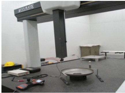
Figure 9: CMM measurement of halfcell.
