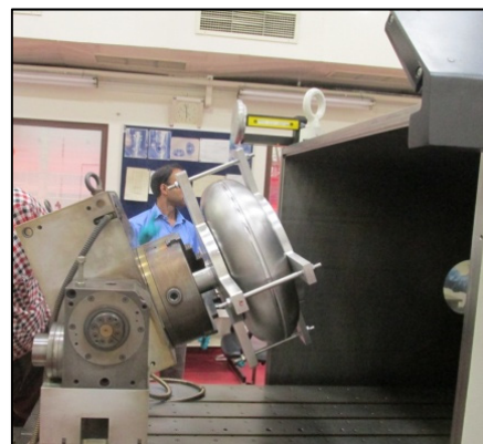
Figure 7: Cavity half cells being put inside EBW machine for equator welding at IUAC, New Delhi.
