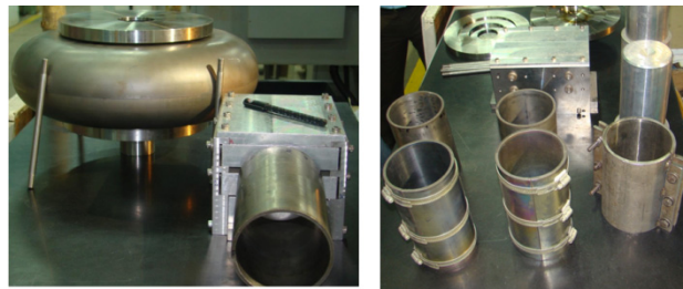
Figure 6: Niobium half cells and beam pipes with fixtures developed for Electron Beam Welding.
