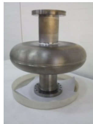
Figure 8: Single cell elliptical cavity after EBW.
