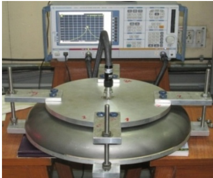
Figure 10: VNA measurement of Niobium Half cell.
