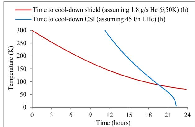
Figure 3: Thermal shield and CSI cool-down duration.
