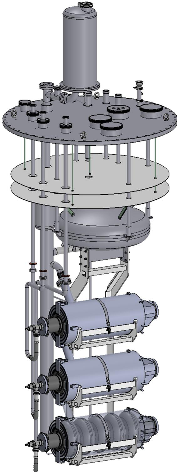
Figure 2: Cavity supports insert (CSI).
