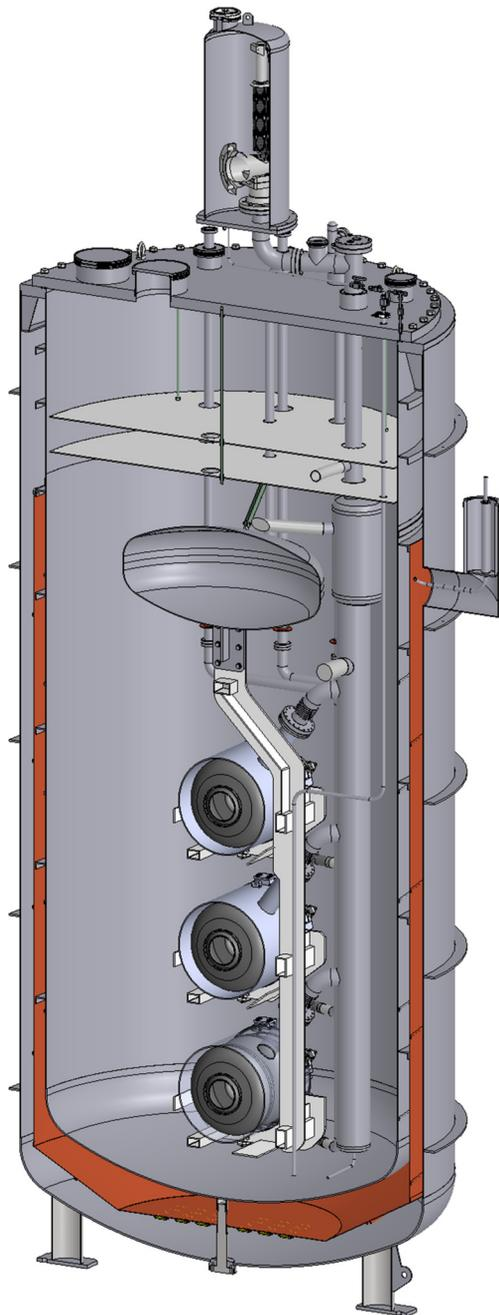
Figure 5: Cryostat section view.
