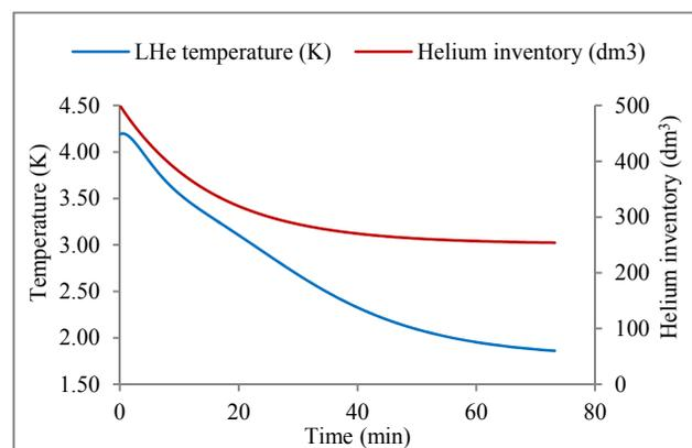
Figure 4: Sub-cooling LHe to 2 K.
