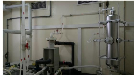
Figure 4: BCP treatment of the HWR cavity.
