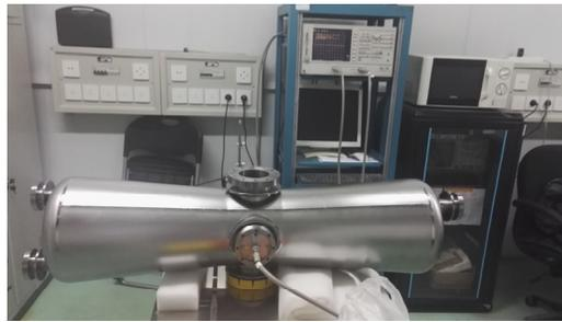
Figure 6: Cavity RF measurements at room temperature.
