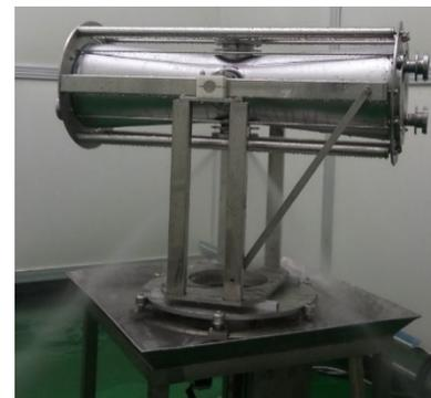
Figure 5: HPR of the  $\beta=0.09$  HWR cavity.
