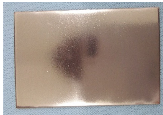
Figure 2: the copper substrate polished by SUBU solution.
