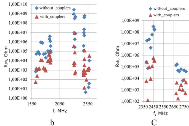
Figure 4:  $Q_{ext}$  (a), transverse shunt impedance  $R_{\perp}$  (b), longitudinal shunt impedance  $R_{\parallel}$  (c), for HOMs in 9-cell cavity without HOM couplers and 9-cell cavity with cylindrical beam pipes and HOMs couplers.
