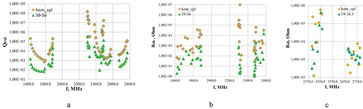
Figure 8:  $Q_{ext}$  (a), transverse shunt impedance  $R_{\perp}$  (b), long shunt impedance  $R_{\parallel}$  (c), for HOM's in 9-cell cavity with corrugated beam pipe and 9-cell cavity with cylindrical beam pipes and HOM's couplers.
