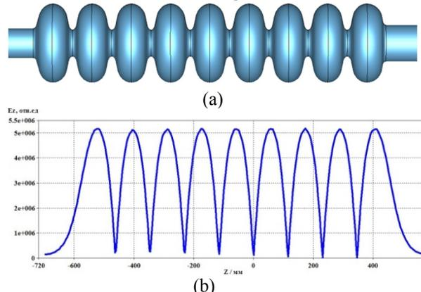
Figure 1: (a) Model of 9-cell cavity with cylindrical beam pipes and (b) electric field distribution for operational mode.
