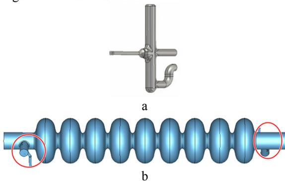
Figure 3: Tesla type HOM coupler (a), 9-cell cavity HOM couplers (b)
