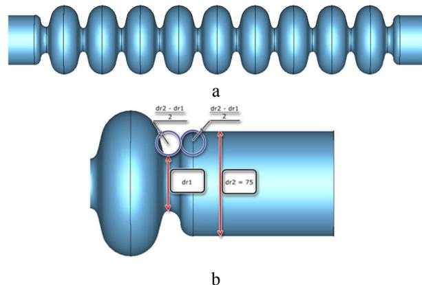
Figure 5: Nine-cell cavity with corrugated beam pipe (a), corrugated beam pipe geometry (b)
