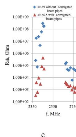
Figure 7:  $Q_{ext}$  (a), transverse shunt impedance  $R_{\perp}$  (b), long shunt impedance  $R_{\parallel}$  (c), for HOM's in 9-cell cavity with cylindrical beam pipes and 9-cell cavity with corrugated beam pipe.
