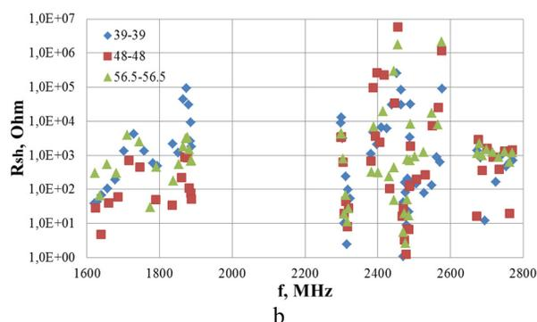
Figure 6:  $Q_{ext}$  (a), shunt impedance  $R_{sh}$  (b) for HOM's in 3 types of 9-cell cavity with corrugated beam pipe and different external radius  $dr1$  (39, 48 and 56.5 mm) Results of EDC of three types of cavities with different radius  $dr1$  comparison are summarized in Table 1.
