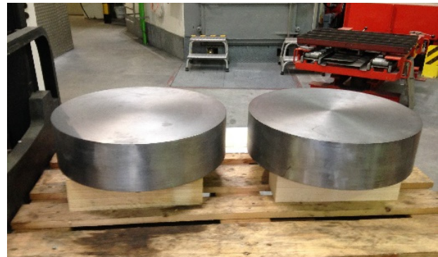
Figure 1: CBMM Large Grain ingots at Heraeus in preparation for the slicing process.
