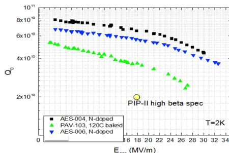
Figure 1: Vertical test results of 650 MHz high beta single-cell cavities for PIP-II.
