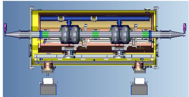
Figure 6: A cryomodule with two 650 MHz 2-cell cavities inside.
