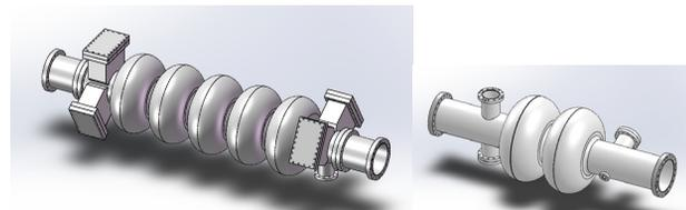
Figure 6: 3D models of the 5-cell and 2-cell 650MHz bare prototype cavities.
