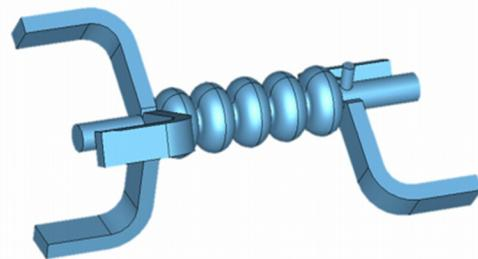
Figure 1: EM design of 5-cell prototype cavity [2].
