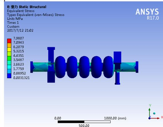
Figure 3: v. M. Stress distribution under self-gravity.
