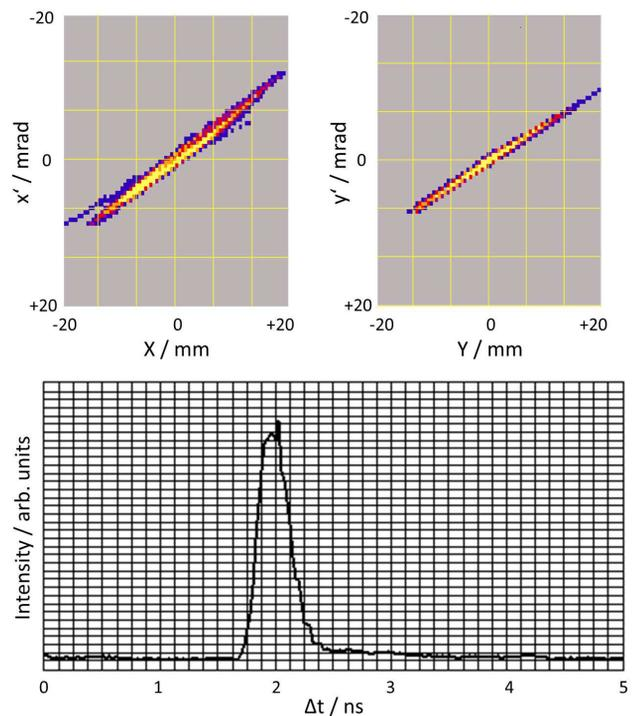
Figure 5: Measured beam emittance (top) and bunch shape (bottom) for accelerated heavy ion beam behind the demonstrator.
