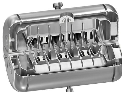
Figure 1: Sectional view of the sc 217 MHz CH cavity [6].
