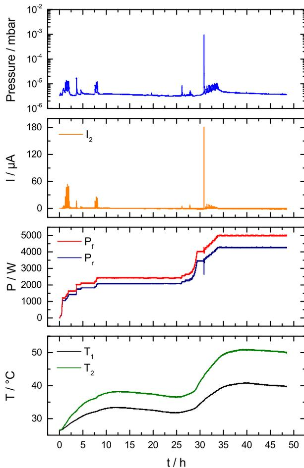
Figure 4: Measuring results of coupler #2 for 5 Hz, 15 ms RF pulses in SW mode up to 5 kW.
