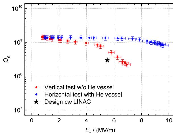
Figure 2: Measured  $Q_0$  vs.  $E_a$  curves at 4.2 K for two different RF tests [7].
