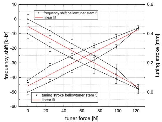
Figure 10: Measured tuning stroke for bellwotuner No. 5.
