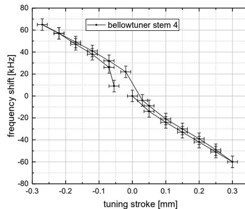
Figure 7: Measured frequency shift for bellowtuner No. 4.
