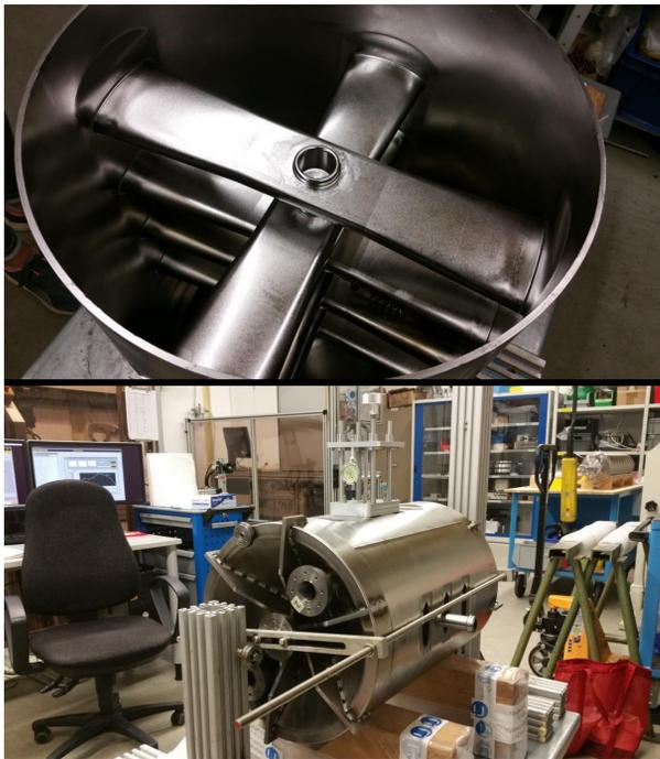
Figure 2: Internal structure (top), measurement setup with temporarily attached end caps (bottom).
