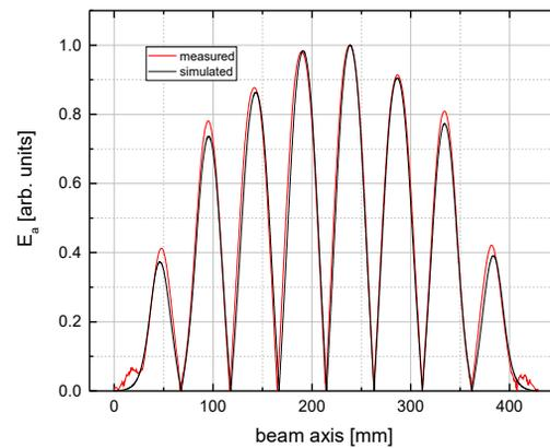
Figure 3: Measured and simulated electric field distribution along the beam axis.
