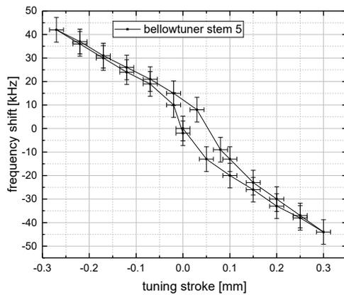
Figure 8: Measured frequency shift for bellwotuner No. 5.
