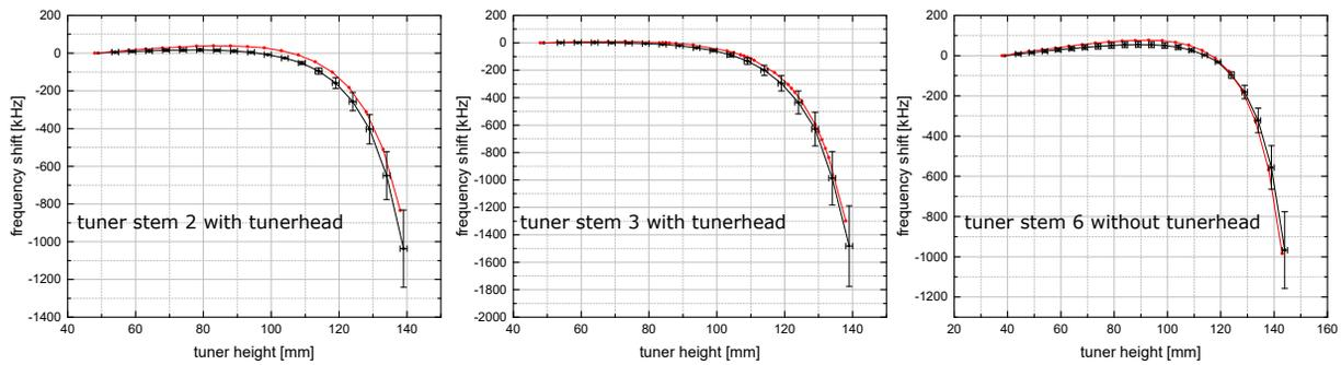
Figure 4: Measured and simulated frequency shift of each static dummy tuner.
