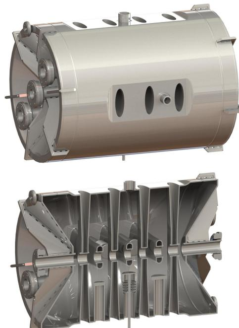
Figure 1: Layout of the sc 217 MHz CH-cavity 2 and 3.
