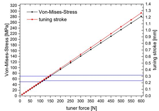
Figure 6: Simulated Von-Mises-Stress and tuning stroke depending on the tuner force.
