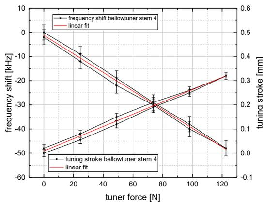
Figure 9: Measured tuning stroke for bellwotuner No. 4.
