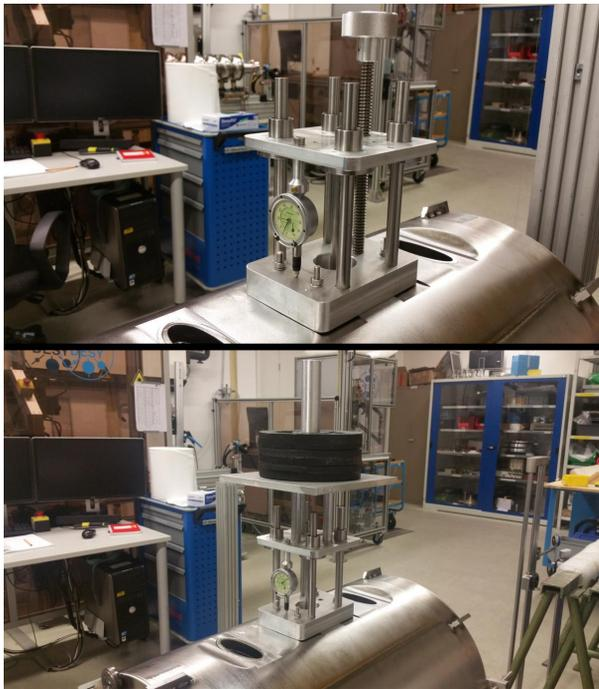
Figure 5: Tuning stroke induced by trapezoidal thread spindle (top), Tuning stroke induced by tuner force through weights (bottom).
