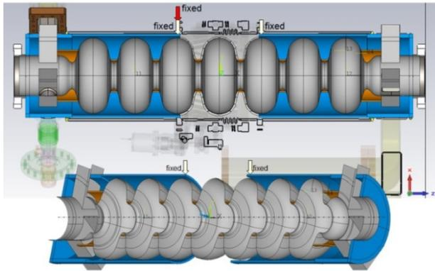
Figure 4: bERLinPro 7-cell elliptical cavity simulation model in provisional helium vessel (stiffening rings are brown).
