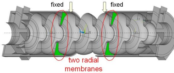
Figure 13: bERLinPro 7-cell cavity in helium vessel with two radial membranes (only end stiffening rings).
