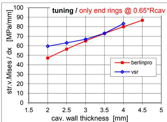
Figure 9: Simulation results maximal stresses with wall thickness variation.
