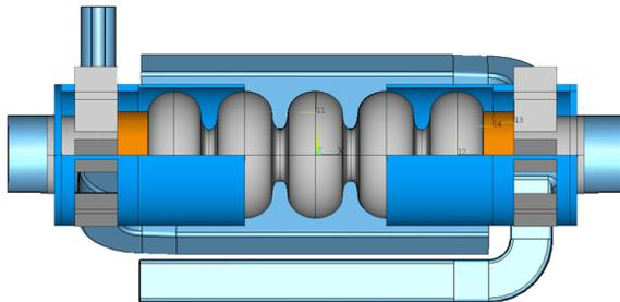
Figure 5: BESSY VSR 5-cell elliptical cavity simulation model in provisional helium vessel.
