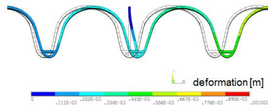
Figure 14: Cavity tuning deformations with transversal radial membrane.
