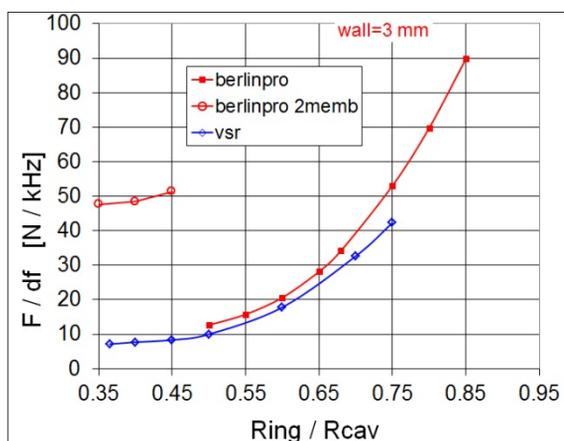
Figure 10: Simulation results of tuning forces with middle rings position variation.
