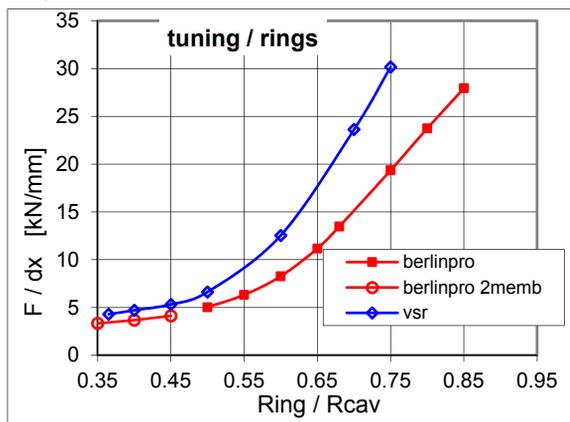
Figure 8: Simulation results of tuning forces with middle rings position variation.
