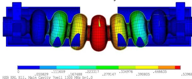
Figure 11: The lowest mechanical transversal mode 1 (84.49 Hz) of bERLinPro 7-cell elliptical cavity in helium vessel with low position ( $R_{ring}/R_{cav}=0.4$ ) of inner stiffening rings.
