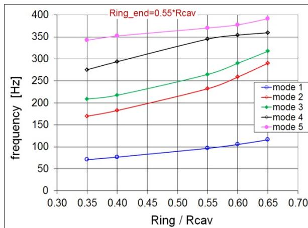
Figure 12: bERLinPro 7-cell elliptical cavity in helium vessel mechanical eigen modes with middle rings position variation.
