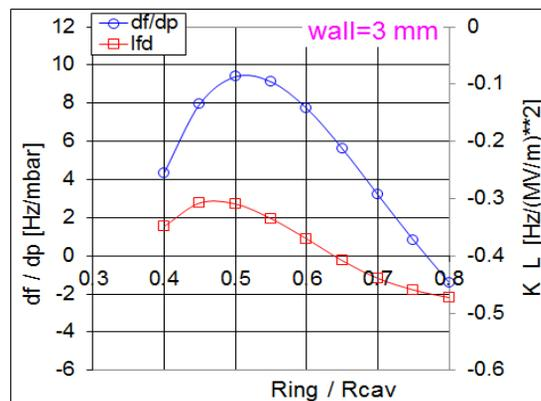
Figure 2: bERLinPro 1300 MHz,  $\beta=1$  middle cell simulation summary (red curve – Lorentz force sensitivity, blue curve – pressure sensitivity).
