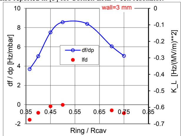
Figure 7: BESSY VSR 5-cell cavity in helium vessel simulation results of  $df/dp$  and LFD with middle rings position variation.
