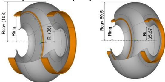
Figure 1: HZB bERLinPro (1300 MHz,  $\beta=1$ ) and BESSY VSR (1500 MHz,  $\beta=1$ ) mid-cell simulation models.
