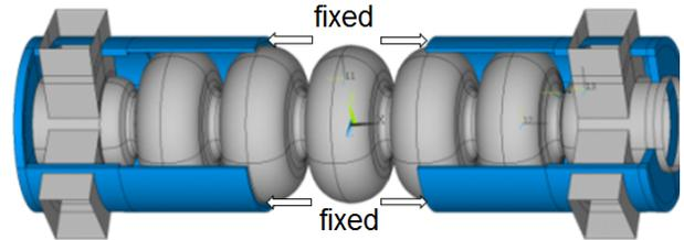
Figure 15: BESSY VSR 5-cell cavity in helium vessel without stiffening rings.
