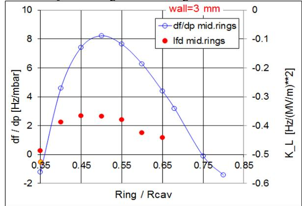
Figure 6: bERLinPro 7-cell cavity in helium vessel simulation results of  $df/dp$  and LFD with middle rings position variation.
