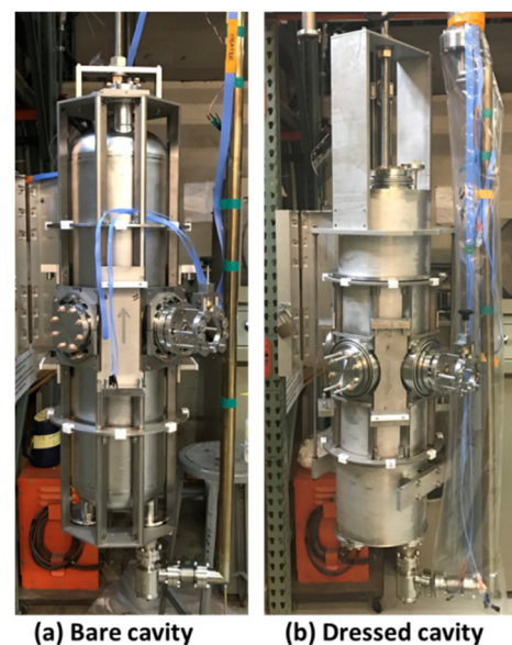
Figure 2: Photograph of (a) the bare HWR cavity (b) the dressed HWR cavity. Both cavities are installed with the handling frames.
