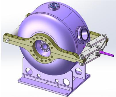
Figure 6: Double scissors type tuner.
