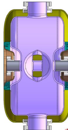
Figure 4: Bellowless helium vessel jacket.
