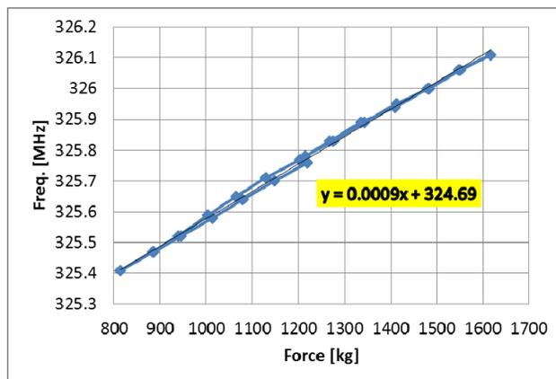
Figure 7: Frequency response vs. tuning force @cooling by liquid nitrogen.
