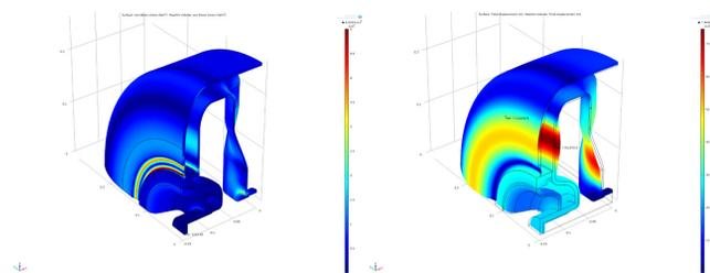
Figure 5: Distribution of stress and displacement with 1bar helium vessel pressure.
