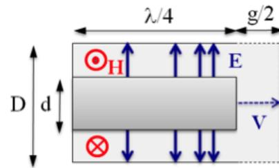
Figure 1: Quarter Wave Resonator (QWR).
