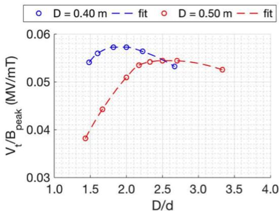
Figure 5: Ratio  $V_t/B_{peak}$  for DQW cavities with different values of  $D$  and  $d$ .
