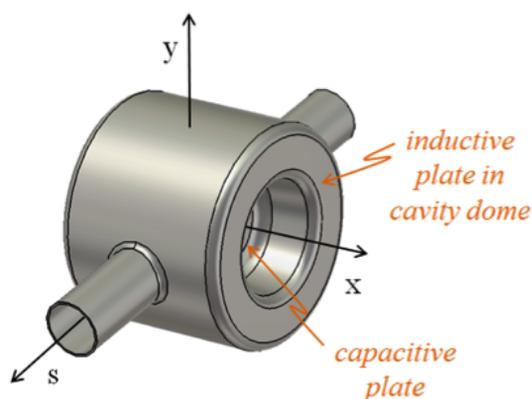
Figure 2: DQW cavity oriented to provide horizontal crabbing kick (x-direction) where s is the beam axis.
