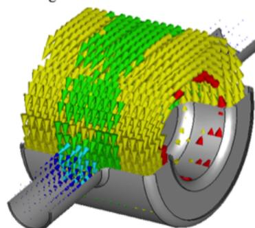
Figure 3: Field distribution in a DQW cavity.
