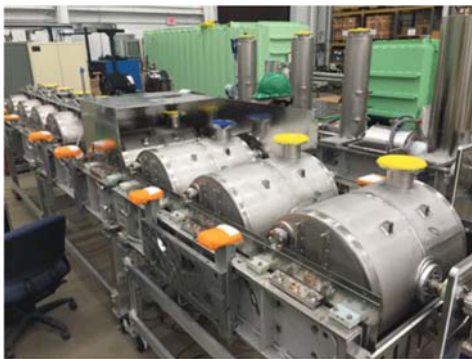
Figure 13: Cold mass for the first HWR cryomodule (SCM501).
