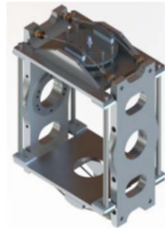
Figure 14: Isometric view of the pneumatic tuner for \beta=0.53 HWRs.
