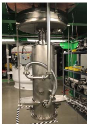
Figure 2: Insert for a Dewar test with a jacketed \beta = 0.085 QWR attached. The helium reservoir can be seen above the cavity.
